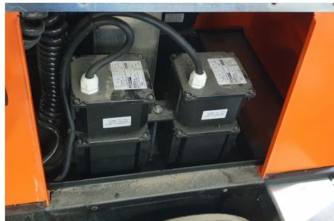
4. Remove the terminal box from the crossbar (but leave the plate behind the terminal box in place). Fit the light fittings to the crossbar. Remove the rectangular (Harting) quick connector from the spiral cable.
