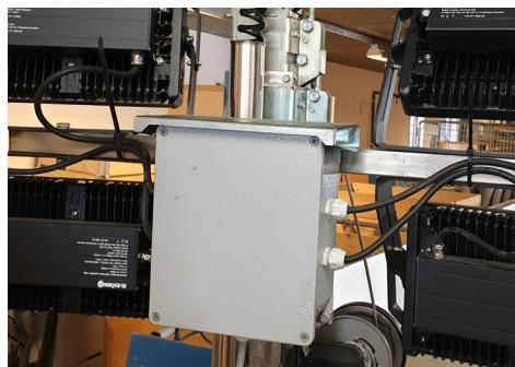
5. Fit a new (female) quick connector to the spiral cable (see photo on right). Check that the correct conductors are connected to the quick coupling. Connect the light fitting cables to the Y connector.
